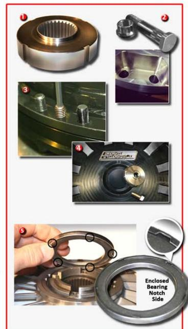
The Stator uses the same sealed bearing on both sides. These bearings have 5 notches on 1 side. The bearings are to be installed with the notched side toward the Stator.
